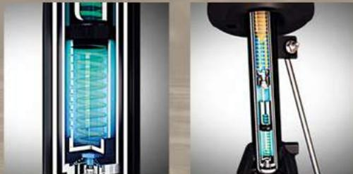
*When big bumps are encountered, the hydraulic cushions keep suspension movement controlled and progressive.*
