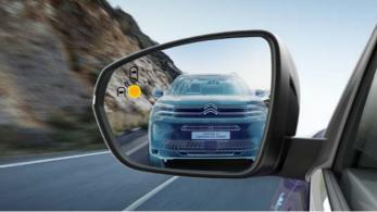
to the driver that there is a vehicle in the blind spots, using an orange LED located in the corner of the door mirrors.
