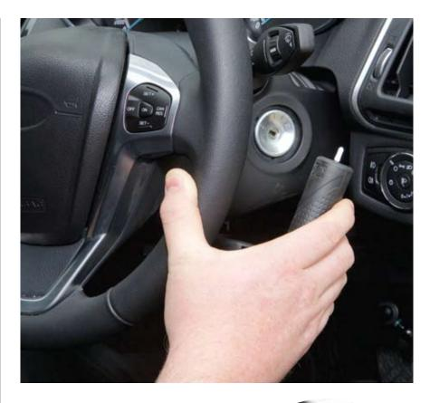
A push/pull device is a good option if you find it difficult to use standard foot pedals to accelerate and brake. You just pull the control towards you to accelerate, then push away to brake. If you think a push/pull device may be right for you, it is important to be aware that push/pull devices are designed for use with automatic gearboxes only.
